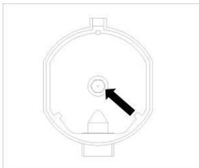
Replacement of burner nozzle: loosen the nozzle with a dedicated wrench(7).Fit the new nozzle according to the required gas type (see table 1 for reference).
