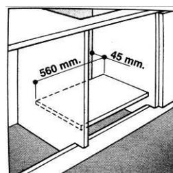
When install hob on a built-in oven without forced ventilation, ensure that have air inlets and outlets to ventilate the interior of the cabinet adequately.
