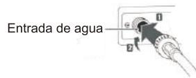
Do not overtighten the hoses. Overtightening can damage the valves resulting in leaking and property damage.
